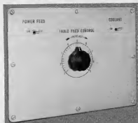
Figure 131A Electrical Controls at Front of Machine
